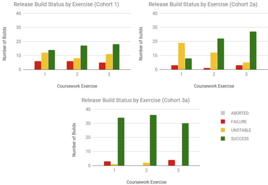
Fig. 6. Total release builds for each build status, grouped by exercise, for the main cohorts.
